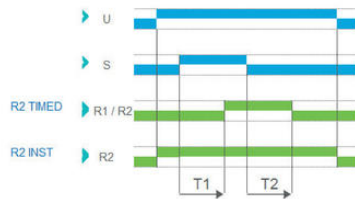
Function Ac - On/Off Delay (Delay on make/break)
